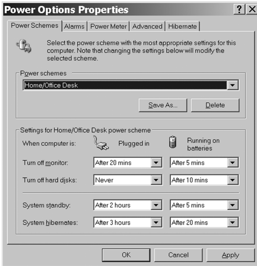
Figure 16-5: The Power Options Properties in Windows' Control Panel enable users to specify power-saving schemes that determine when USB devices must enter the Suspend state.
